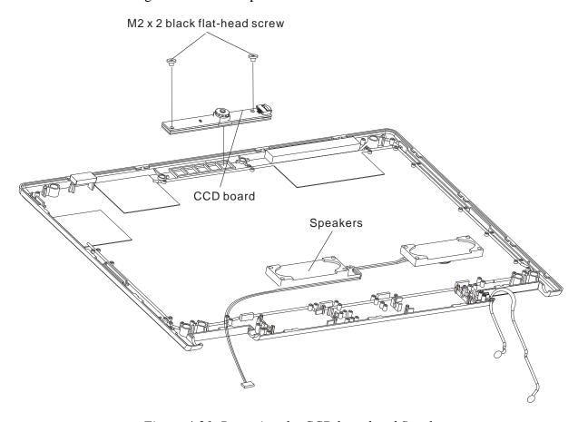
Figure 4-21 Removing the CCD board and Speakers
